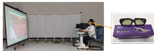
Fig. 4. Lab configuration. The subject wore 3D Active Glasses to watch 3D ME videos. The subject sat at a chair and adjusted the table to the appropriate height. A BenQ TH6370 projector was located under the table and projected to a screen that was placed 3.5 meters away from the subject. The subject used a Bluetooth keyboard to respond. The control computer was placed at the side of the subject.
